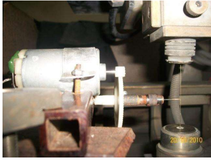
Figure 1: The WEDG-based fabrication process of micro tools
